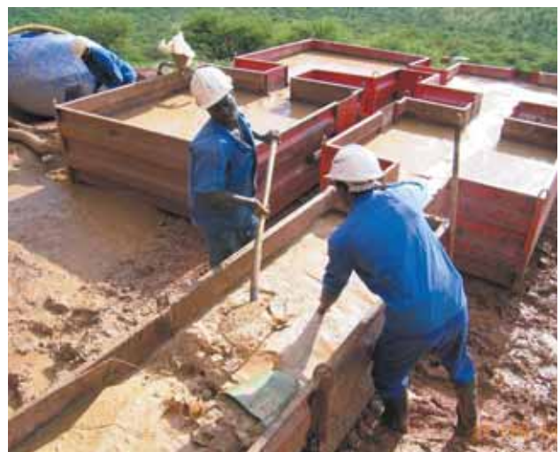
Settling tank system for effective control of solids
