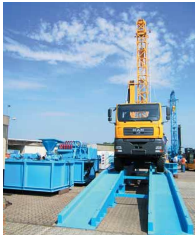
Prakla universal drilling equipment with settling tank system
